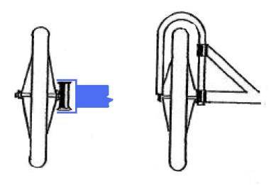
of supporting the wheel is the one to go for. The next decision is means by which the wheel is 'hinged' to the frame. In the case of the one-sided hub arrangement, then this swivel would be incorporated into the hub/axle. In the case of the 'forks' arrangement, the forks themselves can
