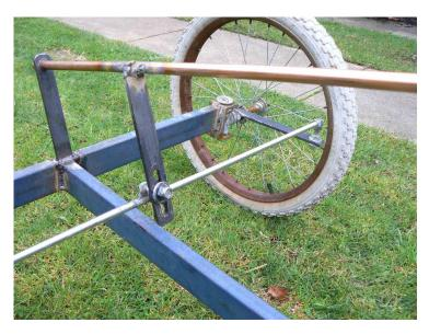
achieved by means of a steering column held in a cycle drop tube. The steering column has an arm attached at 90 degrees. The length of this arm will decide the steering ratio and is the final variable in the whole geometry. Trial and error will be the simplest way of deciding the final on arrangement, but as a
