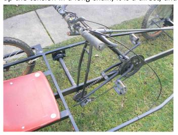
of getting power to the back wheels. The lucky scavenger may even be able to find an adult sized rear axle from a tricycle, which will incorporate a differential and frequently a threespeed or even derailleur type gear attached.
