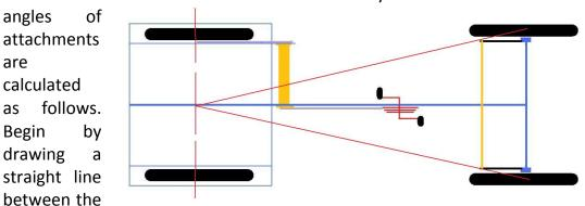
point at which the front wheel touches the ground and the centre of the rear axle. Repeat this process for the opposite side. Selecting a point 150mm or so back down these lines will be the point at which the steering would be linked. If arms are now attached to the forks, which terminate at these points, they may be linked together with swivels at each end and the wheels should now stay in track.
